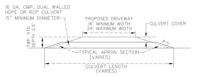
CULVERT LEN. (ft.) = DRIVEWAY WID. (ft.) + 2[((CULVERT DIA. in.+ CULVERT COVER in.)/I2) \* 4]EXAMPLE: I6 ft DRIVEWAY WIDTH, I5" DIA. CULVERT, AND I2 in. COVER CULVERT LEN. (ft.) = 16' + 2[((15" + 12")/I2) \* 4] = 34 ft.
